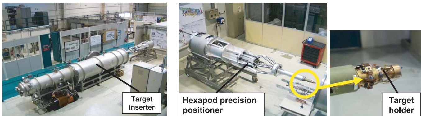
Fig. 8. (Color online) Scale 1 target inserter mock-up in CEA Grenoble – cryogenic technology for thermal control from ambient down to 18 K – left: overall view of the vacuum vessel; right: details of the target positioner and holder.
